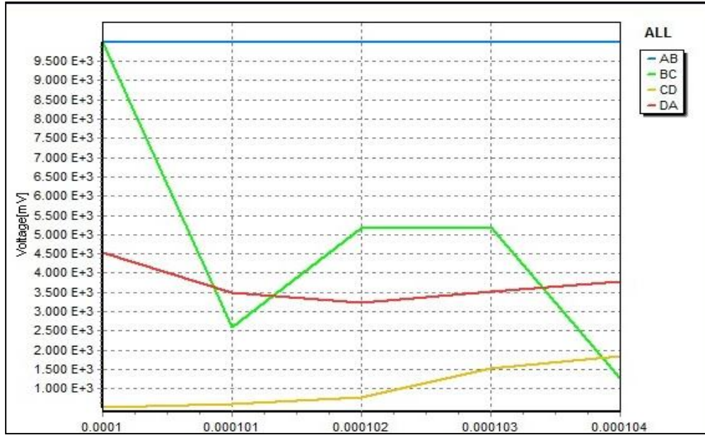
Fig.12 (c) Current-Voltage sweep of ZnS: Cu (1%) thin film on FTO glass by vander pauw method
