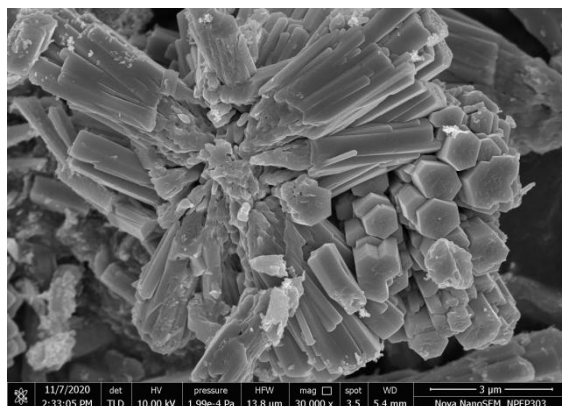
Figure 4: FE-SEM image of ZnO
