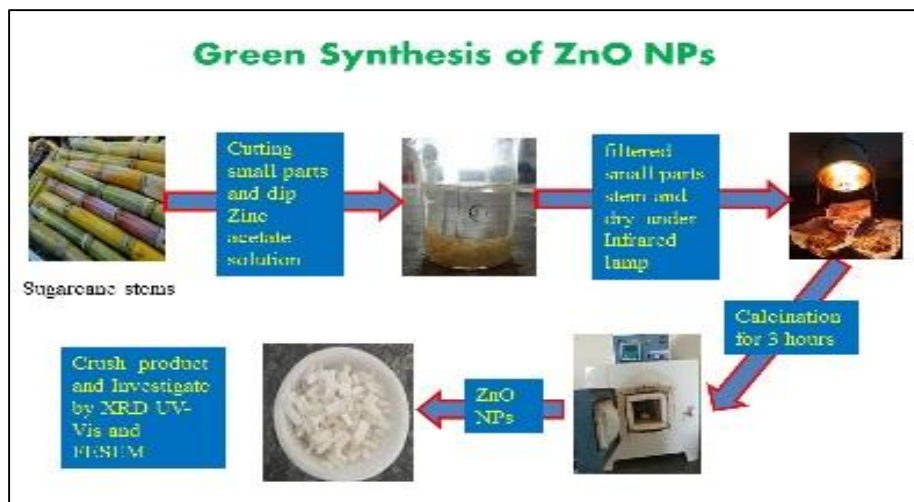
Figure 1: Experimental Scheme of the ZnO NPs by green synthesis using sugarcane stem
